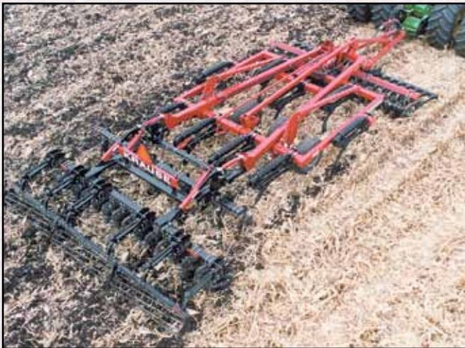
With two full ranks of shanks, none closer than 36" on the same beam, the DOMINATOR® delivers non-stop performance in the highest amounts of tough residue.
